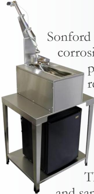
Sonford TC-4 series samplers are designed for use in highly corrosive environments where it is cost effective to eliminate possible refrigerator repair costs and use a disposable refrigerator. This is why the TC-4 models use a stainless steel stand and disposable refrigerator in place of traditional refrigeration.
