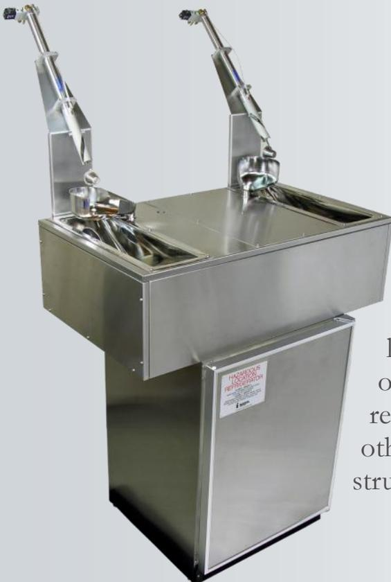
One of the key features of a Sonford Sampler is the unique design of the flow-through reservoir. The reservoir is engineered for constant turbulence in the sampling area, ensuring that no settling of suspended solids occurs. The result is a true representation of the actual flow. The reservoir and all other wetted components before the drain are constructed of stainless steel for longevity and easy cleaning.
