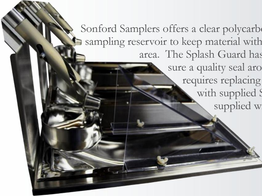
Sonford Samplers offers a clear polycarbonate shield that attaches to the sampling reservoir to keep material within the confines of the sample area. The Splash Guard has a closed cell PVC gasket to ensure a quality seal around the reservoir. Installation requires replacing 4 of the Stainless Steel screws with supplied Stainless Steel studs and using supplied wing nuts to attach the shield.
