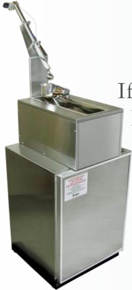
If the atmosphere surrounding the sampler is considered a hazardous location, the TC-3 Explosion Proof series is the right choice. There are only three possible means for ignition with a Sonford Sampler; the refrigerator, solenoid valve and control panel. The TC-3 Explosion Proof series addresses all three areas.
